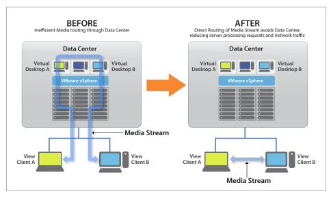
Figure 1: Hairpinning of Real Time Protocol (RTP) media, bandwidth, and the lack of Quality-of-Service (QoS) support for traffic priority were the key inhibitors for VoIP to function properly in the encapsulated desktop virtualization protocols.
